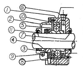
Aligning ring on floating bearing must be located centrally in housing
